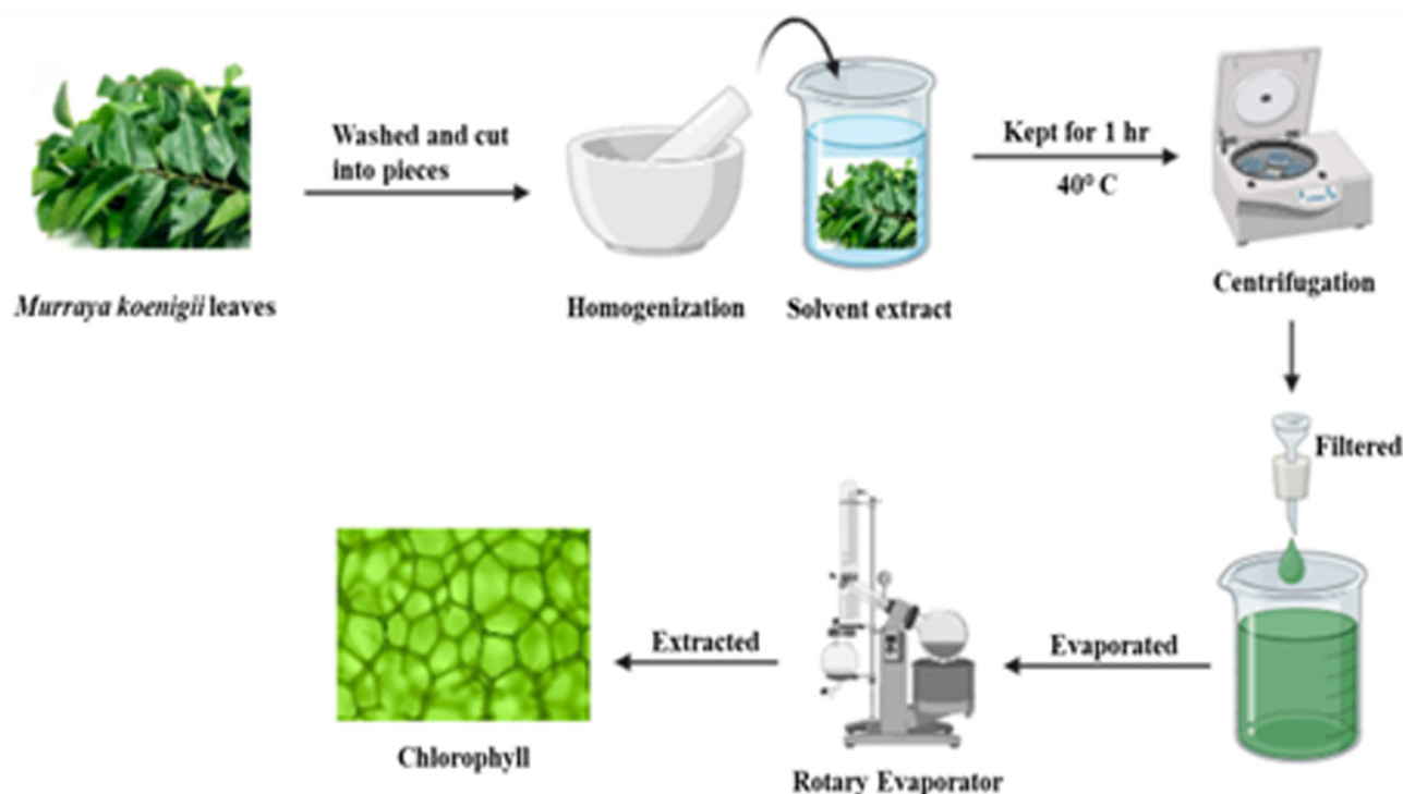
Figure 1: Schematic illustration of chlorophyll extraction process.
